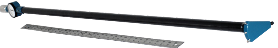
#4 Dorsey/Standard bore gage with 4’ carbon fiber extension housing. The weight is 2½ lbs/1.13kg (less range extensions).
